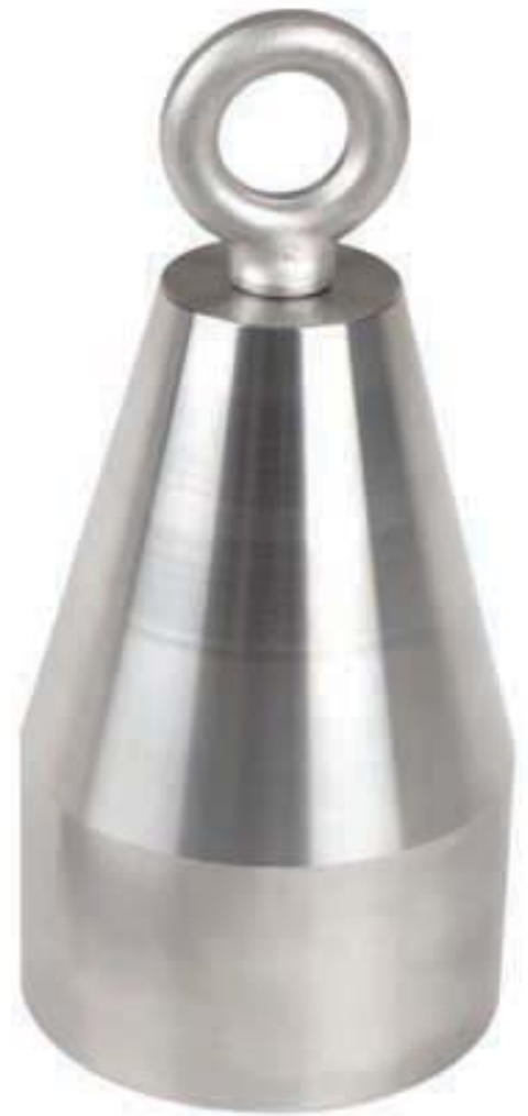
Custom Design Weights 25 kg special shape eyebolt weight to calibrate the load cell on large mixing tanks with lifting bar
